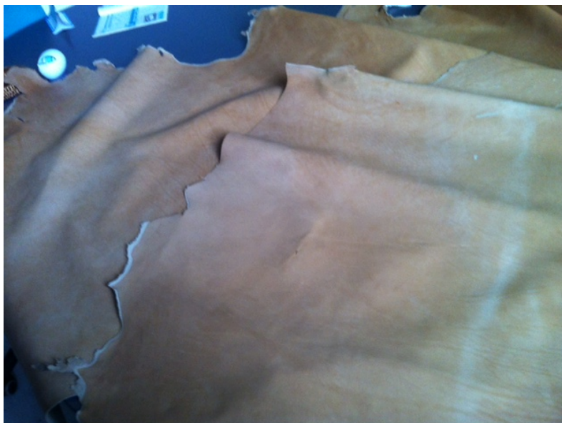
Figure 4.4. Picture of two representative leathers fattened with the natural product Cl-Palmkernel oil FAME, selected for the production of leather products (right in the picture) and with CP44 (left in the picture).
