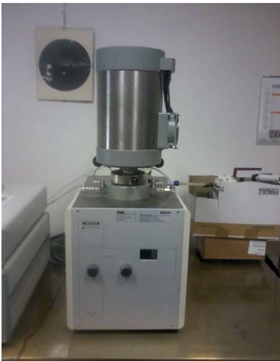
Figure 1: Balance and furnace in TG NETZSCH 409 C.
