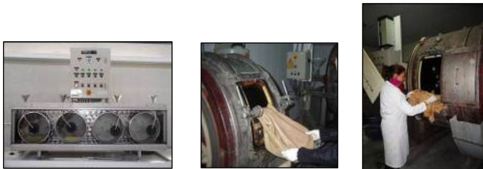
Figure 4. Laboratory, semi-industrial and pre-industrial scale fatliquoring tests (INESCOP-UT Vall d'Uixó facilities)
